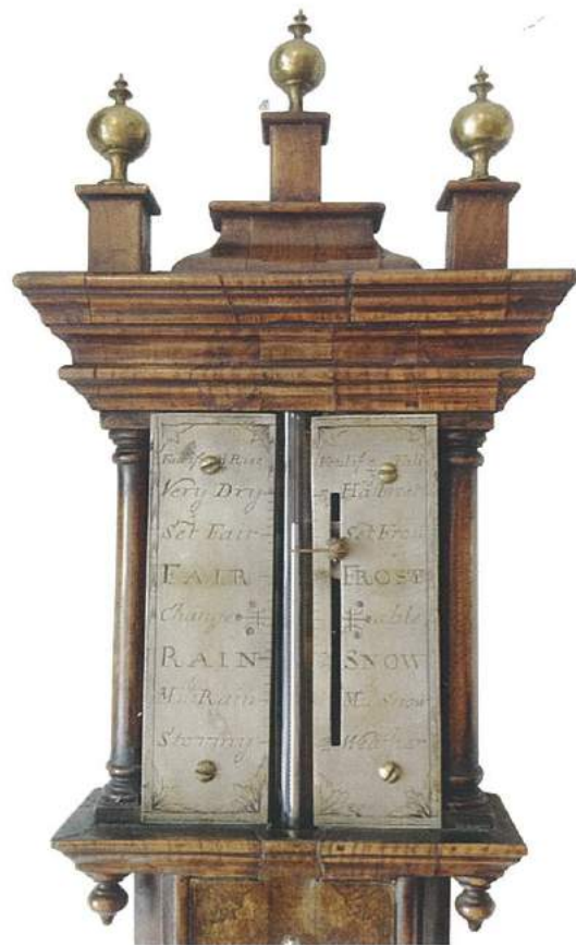
30a. Detail of silvered, engraved scale, Royal Society Scales barometer
