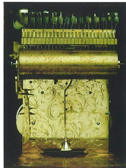
24b. Detail of backplate and musical pin barrel, Robert Henderson bracket clock
