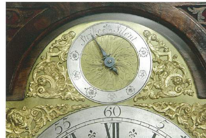
7. Detail of strike-silent dial on a figured walnut bracket clock by Philip Constantin, London, circa 1725
