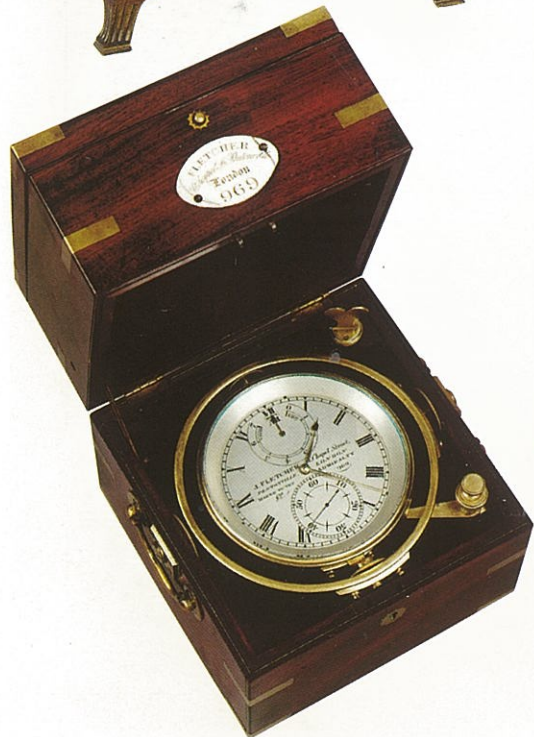
◀ J. FLETCHER, CHAPEL ST., PENTONVILLE, LONDON Maker to the Admiralty No.969 An impressive 8 day Marine Chronometer, the high quality movement with spring-detent escapement and the brass bound mahogany box, in very original condition.
