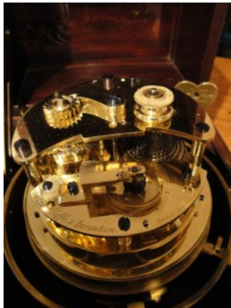
Detail of the interior of Wieland's marine chronometer, with Eiffe's patented temperature compensator. Raffety Antique Clocks
