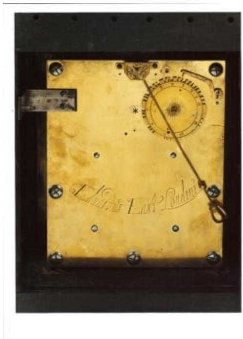
Detail of a backplate on a clock by Edward East, circa 1665-70. This shows the pendulum – a revolutionary technological innovation that first appeared on a working clock in 1656
