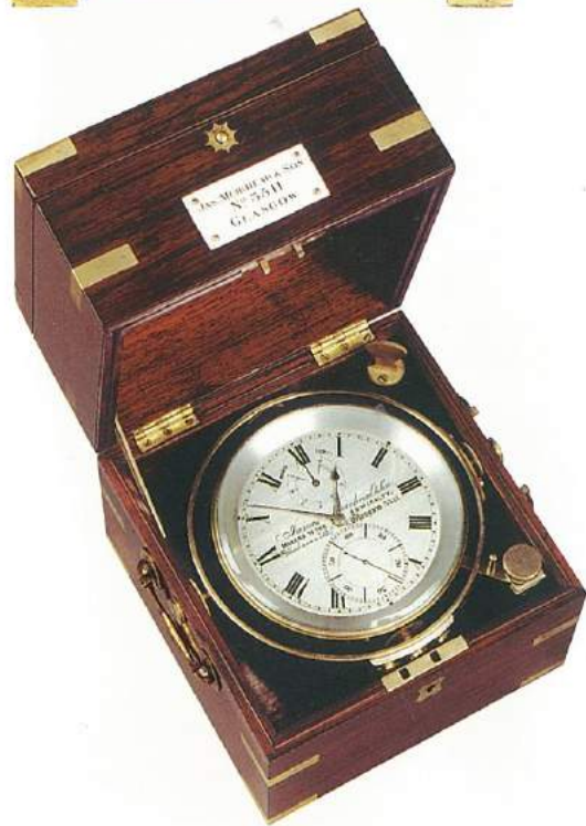
◀ JAMES MUIRHEAD, GLASGOW, No. 3511 A good quality 8-day marine chronometer, the spring-detent movement gimballed within the brass-bound rosewood three tiered case. c.1840. 8 in. square case.
