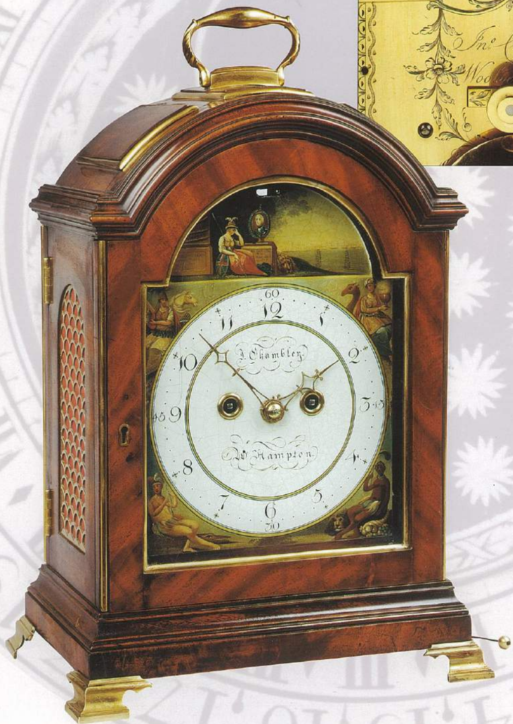
The 8 Day hour striking movement with strike/silent is signed John Chambley, Woolverhampton (sic). Circa 1805 - 1810 Height : 15 1/4 in. (38.5 cm).
